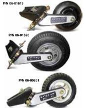
Matco tailwheels use a fiberglass reinforced nylon wheel with an operating load of 450 lbs. It takes over 5000 lbs to fail the wheel and it will hold up in the most rigorous conditions. Can be used with 1-1/4" or 1-1/2" leaf spring. These tailwheels are steerable, and are available with a 6 inch hard rubber solid tire or with 8" Shin pneumatic tire and tube for heavier aircraft. Tailwheel construction is anodized aluminum. Weight: 5 lbs.
