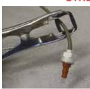
Using the Grommet Stretcher is 2-3x's faster when stretching grommets over fittings and plugs. Improves safety because grommets are continuous.
