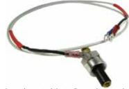
P-Leads are a critical part of the ignition system and their good condition is vital to safety and airworthiness. P-leads are often overlooked and seldom replaced because replacement p-leads are not available from the aircraft manufacturer and materials to fabricate new p-leads are not commonly available. Because most leads are shielded mechanics do not
