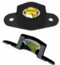
The SK2003A Series Mounts were specifically designed around the latest generation Cessna/Lord J7444-42 Series Mount. The SK2003-14A, -24A, and -42A all have the same flex feature as the J7444-42. They look and install exactly the same as the Cessna/Lord part it replaces using the same fastener length. The SK2003-14A, -24A, and -42A are fixed depth, Non-Adjustable Platemounts. The 50ADJ is adjustable and can be adjusted without removing the cowling for an exact fit.
