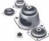
Lord Platform Mounts provide effective isolation against vibration. The contour of the flexing element was developed to provide uniform stress distribution. This, plus high strength bonding and the use of specially compounded elastomers, provides maximum service life. 200 Steel Holder 45 lb.
