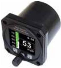
Measures airspeed from 16mph to 250mph and is well suited to slow aircraft due to very good sensitivity and linearity at low air speeds. Includes a flight timer since takeoff. Airspeed units can be set to miles per hour (mph), kilometer per hour (km/h) or knots (kts). Analog tape with programmable ranges for Vs0, Vs1, Vfe, Vno and Vne. Contains a programmable Vs and Vne airspeed alarm output. Records maximum airspeed reached in permanent memory .....P/N 11-15989 .....\$399.00
