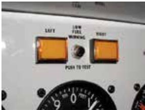
This system gets your attention before you have to switch tanks. When the annunciator light flashes, you will know your precise fuel quantity and also the time to engine shut-down for that tank. HOW DOES IT WORK? - The optical fuel sensor is a non-contact sensor mounted in a single hole in the fuel tank. It operates by bouncing a beam of light into the sensors lens. If it is reflected back into the sensor, there is
