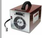
From Concorde, a portable, light weight unit designed to provide the operator with an economical, easy, and accurate means for capacity testing aircraft batteries. Fully automatic testing for 12 Volt AND 24 Volt lead acid aircraft batteries. Powered by the battery being tested - No AC power required. Constant current load adjustable in 1.0 Amp increments 10 to 55 Adc. 50 mv voltage resolution. 10 LBS / 4.5 KG Length 12" (30
