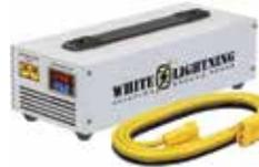
Clean, stable, airframe power specifically for the needs of the E/A-B aircraft. Output fixed at 14.25VDC, up to 35A maximum continuous power. Ideal for cockpit database and EFIS updates, flight planning, powered preflight, procedures training, and general maintenance. Includes an Airframe Interface Kit to permanently wire a quick-connect polarized receptacle to the aircraft's main electrical bus. Detachable, replaceable 6' output cable included. Fully protected operation with automatic recovery.
