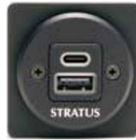
**Features:** • Dual 3.0 amp charging ports, USB-A and USB-C • Blue LED lighted front • FAA certified to TSO-C71 • Designed and built in the USA • Cylindrical shape for easy, drill-in panel installation • Shielded to prevent any added RF noise in comm radios • 5-year warranty backed by Appareo
