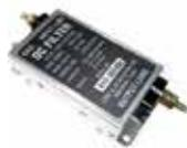
100 amp filter (FEED THRU) (Fail Safe Design) attenuates both low and high frequency, (10hz to 30 mhz) of EMI-RFI noise generated from the aircraft's alternator systems to the aircraft's dc buss. This filter, (100 amp Fail Safe design) is used by OEM aircraft manufacturers to attenuate 100% of the on board noise before it penetrates the aircraft's dc buss. The filter is FAA- PMA pending for certificated aircraft but can be used on experimental aircraft.....P/N 11-04850 .....\$349.95
