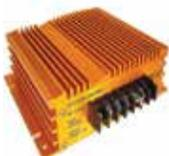
With this TSO-C71 DC to DC Converter you can operate 12 Volt Radios, GPS's, and Electronic Devices in a 24 Volt Aircraft. Size: 6.0"W x 5.0"D x 1.75"H. Weight: 1.5 lbs. Color: Gold Anodized. Material: Aluminum Extrusion. P/N 11-03309 .....\$449.95
