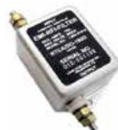
70 amp filter attenuates EMI-RFI noise generated from alternator, generator systems, gear motors, blowers for a/c systems and other higher current noise sources. Can be used to filter the aircraft's avionics buss to filter RF, NAV, GPS, as well as other navigational equipment. The filter is FAA- PMA for certificated aircraft as well as for experimental aircraft.....P/N 11-04849 .....\$328.00
