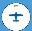
An approved anti-collision strobe light system must project light 360° around the aircraft's vertical axis. One or more strobe lights can be used.
