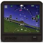
D3 lets pilots supplement their unreliable legacy instrumentation with an affordable, portable electronic attitude indicator that works. The D3 features the same reliable, proven AHRS engine from Dynon's bestselling panel-mounted products for experimental, light sport, and type certificated aircraft.
