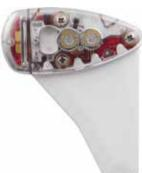
skyBeacon is a 2020 compliant, near zeroinstall, Class B1S ADS-B UAT transmitter and WAAS GPS integrated into a wing tip position light. The power transcoder decodes replies from legacy Mode C transponders. 14 CFR §91.227 compliant. Smart phone configurable over WiFi. skyBeacon is a revolutionary new way to equip ADS-B. Simply replace your existing navigation light with skyBeacon and you are ADS-B compliant for 2020.
