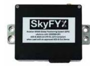
SkyFYX combines a high precision WAAS GNSS sensor with an integrated RAIM processor. Resilient against jamming, spoofing and GPS range errors—SkyFYX provides reliable navigation in challenging environments. SkyFYX is the most affordable ADS-B rule-compliant position source companion for the echoUAT ADS-B transceiver. The Sky-FYX meets the performance
