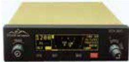
The STX 360 Sentinel is a 978 MHz UAT ADS-B unit with a built-in Mode A/C transponder. The STX 360 can easily be installed in the same space as an existing transponder, simplifying the installation. The STX 360 has an internal diplexer that allows both the transponder and the UAT to share a single antenna.
