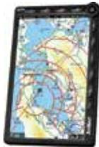
**Fully Portable:** A brilliant 7" display, with built-in battery and GPS, only 0.8" thick. EKP V is slim and light, yet very powerful: with built in u-blox 5 GPS receiver, built-in battery and speakers.
