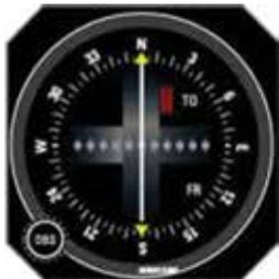
The KI203, KI208, KI204, & KI209 indicators feature an internal VOR/ LOC converter and are compatible with the KX155 transceiver. The KI203 & KI204 have rectilinear meter movement, while the KI208 & KI209 feature pivot needle action. The KI206 has rectilinear meter movement and works with the KX165 & KNS80. The KI209 includes GPS interface capability. Size: 3.125" x 8"D; Weight: 1.5lbs.
