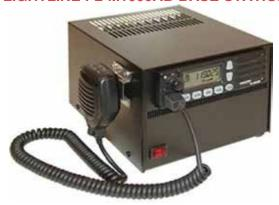
FL-M1000A Air Band Land Radio installed in an Astron Base Station. The FL-M1000A is an Air Band Land Mobile Radio designed for land vehicles, or base station use, not for Aircraft. The radio can be operated with Hand Microphone or Headset. You can choose audio output from External Speaker and/or Headphone. The radio has various built-in Scan functions.
