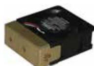
The SAFE 128 is an axial fan that is designed to attach directly to an avionics unit's cooling port. Providing a nominal 20 CFM (no load) of cooling air. The SAFE 128 provides an alert output whenever the fan RPM drops below a preset level. **Specifications:** • Voltage: 28 Vdc • Current Draw: 100mA nominal <250mA Startup • Size: 2.36" x 2.87" x 1.44" • Weight: .25 lb. • Certification: PMA,DO160D • With Fault Detention ..... P/N 11-08019 ..... **\$285.95**
