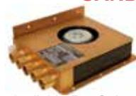
The ACF528 is a FAA-PMA'd five port cooling fan that produces cooling air for one to five avionics units. Supplying up to 20 cubic feet of air per minute at 28 Vdc, the ACF528 can easily cool an entire stack of avionics. The ACF528 uses a brushless blower motor to provide years of reliable RunQuiet™ operation. **Specifications:** • Operating Voltage: 28Vdc • Current Draw: 480mA (850mA startup) • Size: 5.13" x 6.77" x 2.1" • Weight: 1.18 lbs • Certification FAA-PMA: DO160C
