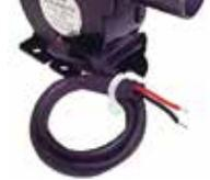
**Specifications:** • Light Weight: 52 grams, 0.115 lbs • Enclosure: Aluminum, (powder coated) • Vdc, amperage: 12 = 10.2-15.8Vdc, 0.320ma • Vdc, amperage: 24 = 18.2-28.5Vdc, 0.300ma • 1 port = 5/8 inch x 1.0 • Max Static pressure: H2O = 0.64 • Max Air Flow: 6.7 CFM • Universal Mounting Bracket: (4) (mt)(h) • Operating Temp: -55C to +70C • FAA-PMA (pending), 6-30-08 • Ultra-Small Size: 2.0H x 1.00W x 2.0L • Easy Installation: (4 x 6-32) • 1 year Limited Warranty
