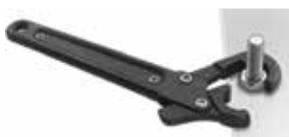
You'll have the advantages of an open-end wrench, plus the convenience of ratchet action. The jaws snap open to slip onto fittings and fasteners; then, they close tightly for ratcheting. Wrenches require a 30 degree handle swing to turn a fastener. All are made of hardened steel with a black finish.
