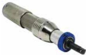
The MD1F35H is an adjustable driver with a range of 5 to 35 lb. in. Body is constructed of steel and anodize aluminum, has a CNC machined knurled grip and 1/4" male drive and comes packaged in a plastic box. The MDP1F35 is a preset model ideal for repetitive assembly operations.
