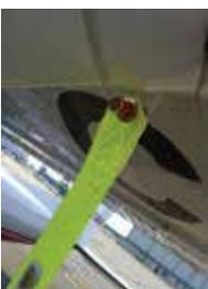
Fuel flow to your aircraft's engine can be compromised by insects or debris entering fuel tank vents. This remove-before-flight Fuel Vent Screen prevents contaminants from obstructing or contaminating the fuel system. The attached foot-long, florescent, and weather-resistant reflective streamer stands out equally well in daylight or darkness under all weather conditions, so it won't be forgotten during your pre-flight. Fits Cessna piston engine aircraft. Inside diameter of PVC sleeve is 0.365"
