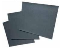
3M<sup>™</sup> Wetordry <sup>™</sup> Abrasive Sheet 413Q is an abrasive sanding paper constructed on a light, A-weight paper backing and features a waterproof resin bonding to help prevent heat buildup. The silicon carbide abrasive and waterproof backing make this paper an ideal product for sanding applications such as paint prep, sanding, sealer sanding, and solid surface finishing. This will produce satin-smooth finishes on metal and other doped, lacquered, or enameled surfaces.
