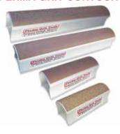
These user friendly sanding blocks are made from extruded, anodized aluminum. The 32mm (1.25") Radius Curve is covered on the external and internal radius with Tungsten Carbide abrasive sheets. The Contour Blocks come in either the Coarse (60US grit approx.) or Fine (120US grit approx.) Small block is 5.5" long and large block is 11" long.
