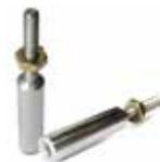
Use these stainless steel extensions for moderate length adjustments to stock length controls. Stocked with 1 male & 1 female threaded end. The extensions provide the required increase in control length when threaded approximately half way onto the control. Furnished in 2", 3", 4", 5" and 6" lengths. All extensions have 10-32 threads. To order, add -2, -3, -4, or -5 to Dash number for length...P/N 10376 .....
