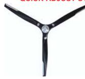
The Quick Adjust System Ivoprops allow you to adjust the pitch on the ground in a matter of seconds by turning the screw adjustor in the center of the prop. Specify aircraft and engine make and model, and propeller diameter. • Magnum Ivoprop (5.5" cord, 58" to 76" diameter) is bible breastern and specific specif a high-horsepower version for engines up to 700 HP.
