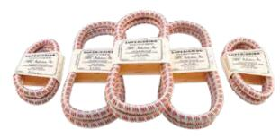
An endless elastic ring composed of multiple strands of natural rubber, wound into a circular skein. Braided cover is high grade yarn. Manufactured to meet specification MIL-C-5651B, Type II. Shock cord is used in landing gear to reduce shock transmitted to fuselage while landing and taxiing and on other shock mounting applications. Color coded to insure fresh stock.
