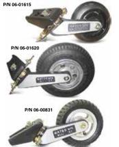
Matco tailwheels use a fiberglass reinforced nylon wheel with an operating load of 450 lbs. It takes over 5000 lbs to fail the wheel and it will hold up in the most rigorous conditions. Can be used with 1-1/4" or 1-1/2" leaf spring. These tailwheels are steerable, and are available with a 6 inch hard rubber solid tire or with 8" Shin pneumatic tire and tube for heavier aircraft. Tailwheel construction is anodized aluminum. Weight: 5 lbs.
