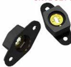
The SK2003A Series Mounts were specifically designed around the latest generation Cessna/Lord J7444-42 Series Mount. The SK2003-14A, -24A, and -42A all have the same flex feature as the J7444-42. They look and install exactly the same as the Cessna/Lord part it replaces using the same fastener length. The SK2003-14A, -24A, and -42A are fixed depth, Non-Adjustable Platemounts. The 50ADJ is adjustable and can be adjusted without removing the cowling for an exact fit.
