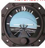
is another variation of our standard 5000B model. It includes inductive pickoffs that generate the signals necessary to drive an autopilot. The intuitive display has a moving horizon mask that indicates the position of the aircraft's wings in relation to the natural horizon. This attitude information is passed along to the autopilot system.
