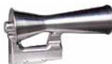
This "super venturi" is similar in appearance to the 4" venturi but with redesigned air passages and a recontoured, long (11-1/4") horn. It pulls enough vacuum to operate a gyro horizon, directional gyro and a turn/bank. Must be used with a suction regulator P/N 15052 ..... ---
