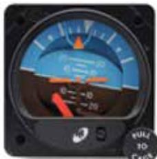
The Mini Gyro offers big features in a compact package. At half the cost of the competition, the Mini Gyro not only saves panel space, but also time and money. An ideal standby instrument, this TSO-approved indicator has 10-32 volt DC operation and is an attractive alternative to vacuum systems. It features unique LED lighting selectable to 5, 14 or 28 volts. Remote emergency power supply available for this indicator (P/N 11-05540).
