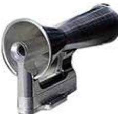
This venturi develops 4" Hg suction from double-throat venturi and 10" long horn. Used to operate a directional gyro or gyro horizon. When operating a directional gyro there is sufficient capacity to also operate a turn/bank. All aluminum construction. May require a suction regulator. Wt. 0.9 lb. P/N 15050 ..... ---
