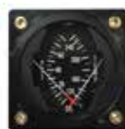
DUAL OIL PRESSURE OIL TEMPERATURE 0-80 PSI/100-260°F P/N 2DA3MM.....
