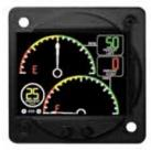
The GEN-2 Fuel Gauge is designed to work with either one or two industrystandard 0 – 5 volt probes, as is common with capacitive probes, or with either one or two industry-standard resistive probes, which are often referred to as float-style probes. Instruments are offered for both 2 1/4" and 3 1/8" panel cutouts. The current fuel level is shown as a standard dial for one or two tanks, along with a digital representation for each tank.
