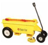
This Start Pac GPU is designed for ground use to perform repeated engine starting functions on the ramp. The 3326XL Special unit is designed for electrically started standard and voltage sensitive turbine engines. Due to the size of the battery bank in this Start Pac engine starting unit, when the unit is depleted, recharge time may be as long as 7-9 hours.
