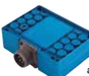
The highly efficient TC120 DC-to-DC Converter produces 120 watts of power from an aircraft’s 28 VDC input. Engineered to run cooler and featuring a fanless design, the TC120 saves energy and reduces weight. It produces enough energy to power electronic equipment throughout the aircraft, including in-seat, cabin and cockpit power applications .....P/N 11-14449 ---
