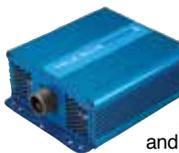
DC-to-AC static inverter produces 115 volts at 60 Hz for 500 watts of “wall outlet” power from an aircraft’s 28 VDC input. Has the same connector and footprint of legacy designs, plus overload and short-circuit protection up to 150 percent of the rated load. Supplies
