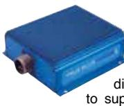
A lightweight power converter that translates a 20 to 36 VDC input to a 115 VAC output at 60 Hertz and provides 250 watts (VA) of power. The alternating current output is defined as a pure sine wave with less than 2% of total harmonic distortion for clean, noise-free, harmonic-free power to supply nearly any common commercial or consumer
