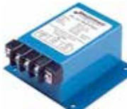
This classic DC to AC solid-state “peanut” inverter provides a reliable source of 26 volt, 400 Hz, AC power. Versatile, compact and lightweight, it is ideal for use with Stormscope bootstrap and multifunction display installations. Input: 11-40VDC @ 0.75 amp. Output: 26 VAC, 400 Hz, Single Phase, 10 volt-amperes .....P/N 11-07062 ---
