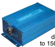
The TI1200 DC-to-AC static inverter produces 115 volts at 60 Hz for 1200 watts of “wall outlet” power from an aircraft’s 28 VDC input. Lighter and smaller than competing inverters, the TI1200 has the same connector and footprint of legacy designs, plus overload and short-circuit protection up to 150% of the rated load.....P/N 11-10743 ---
