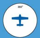
approved anti-collision strobe light system must project light 360° around the aircraft's vertical axis. One or more strobe lights can be used.
