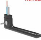
The Fully Integrated Probe, containing an Air Data Computer and an Attitude and Heading Reference System, replaces any AN5812 Pitot Probe. The Digital Pitot Static Probe provides: Airspeed, Altitude, Vertical Speed, Angle of Attack, Outside Air Temperature, Attitude, Heading and Clock - all visible on one or more T3000 skySuite instrument displays.
