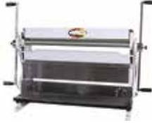
These Sheet Metal Roller Presses have 6 adjustable hardened fingers, spring loaded sheet hold-down, heavy cast iron frame, grooves for wire rolling, 1 1/4" slip rolls, adjustable back gauge. Works up to 20 gauge sheet metal. Stand not included but available for the 30" Roller only.
