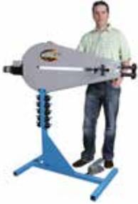
Heavy Duty Power Bead Roller, works off 110v gear drive motor and has a 43" throat depth with an adjustable fence and includes floor stand, die rack, 2 step dies, 2 bead dies and a 45 degree tipping die.
