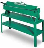
Versatile, economical hand brake designed for straight forming of mild steel in thicknesses of 22 gauge & lighter. Made in the U.S.A by Tennsmith. Bends material up to 48" wide. Wts: brake: 280 lbs. Optional stand: 95 lbs. Ideal for bending materials used in light aircraft construction. Shipped direct to you from factory in Tennessee. Model S48-22 hand brake
