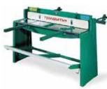
Tennsmith squaring shears offer precision shearing and rugged construction. These shears feature traction, ground alloy tool steel blades to prevent material movement during shearing. Will shear material up to 16 gauge mild steel and up to 20 gauge stainless steel. Both blades are adjustable and back gauge gives highly accurate readings. Wts: Model 36: 700 lbs.
