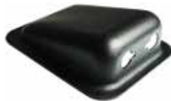
2 HOLE SURFACE MOUNTED MIC & PHONE JACK HOUSING Mounts flush to any flat surface. Heat-treated aluminum with a powder coat finish. Jacks not included. (See electrical section).
