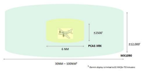
NM, the closure time increases to 5 minutes. The altitude window for detection is extended to ±12,000 to ensure rapid descending/ascending aircraft are detected with advanced warning. For example; an aircraft climbing at 6000 FPM will only take 2 minutes to reach your altitude with a 12,000 foot separation.
